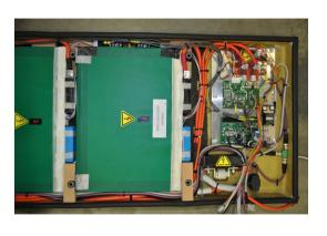
Thirty-five Kokam 100 Ah lithium ion polymer cells, Elithion Battery Management System (BMS).
