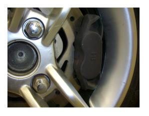
Trev uses motorcycle disk brakes on all three wheels.
