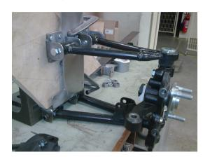
Unequal arm double wishbone suspension, designed to minimise track changes.
