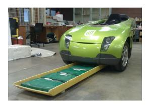
The battery tray is made from 15 mm thick polypropylene honeycomb with kevlar skins.
