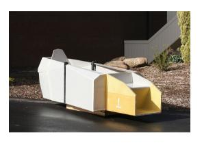
20 mm thick aluminium foil honeycomb boards with fibreglass skins. Floor and front compartment reinforced with keylar.
