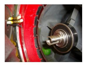
Trev has a Vectrix brushless motor with a Semikron IGBT power stage and a custom control stage.
