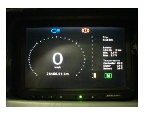
Information was displayed on a 7" LCD screen from an AMOS 3000 12 V fanless PC with a solid-state drive, running TinyCore Linux. Software was written in Processing.
